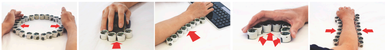
Figure 4 SwarmHaptics: Haptic display with swarm robots [10].
