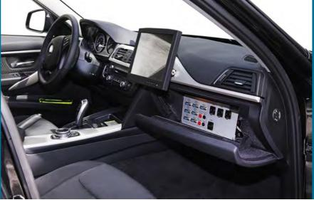
The test vehicle that Fraunhofer uses for researching vehicle-environment networking applications, mutual driver-assist systems, and driving environment modeling is named VICTOR. The vehicle has several antennas with which it receives not just GPS and LTE signals, but also ITS-G5 signals (the WLAN standard for vehicles). Laser scanners and two side-looking radar systems provide the mechanism for recognizing obstacles and other drivers.
